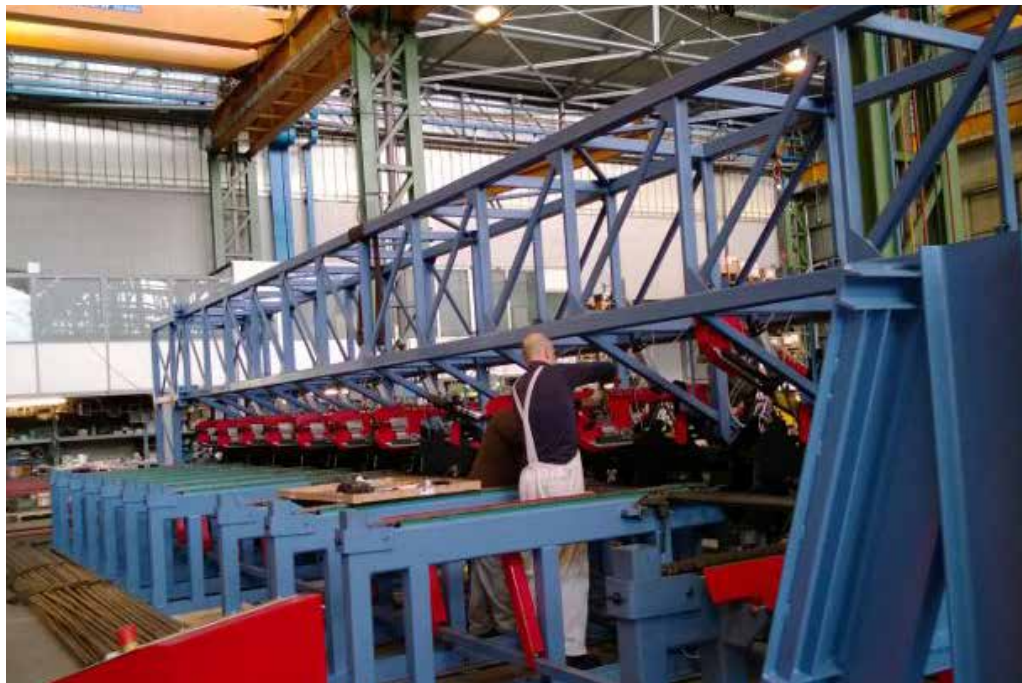
11 teste automatiche per taglio tiranti \varnothing 10-120 mm da 1 a 12 m - 11 automatic heads for rebar cutting, \varnothing 10-120 mm, lengths from 1 to 12 m
