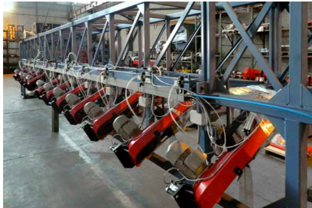
11 teste automatiche per taglio tiranti \varnothing 10-120 mm da 1 a 12 m - 11 automatic heads for rebar cutting, \varnothing 10-120 mm, lengths from 1 to 12 m
