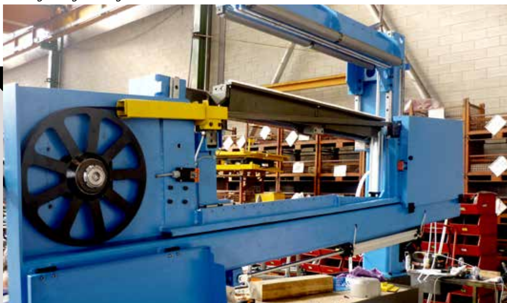
Taglio pannelli in resina 1.250 x 300 mm allineamento gancio eccentrico Resin panel cutting 1.250 x 300 mm with cam lock alignment
