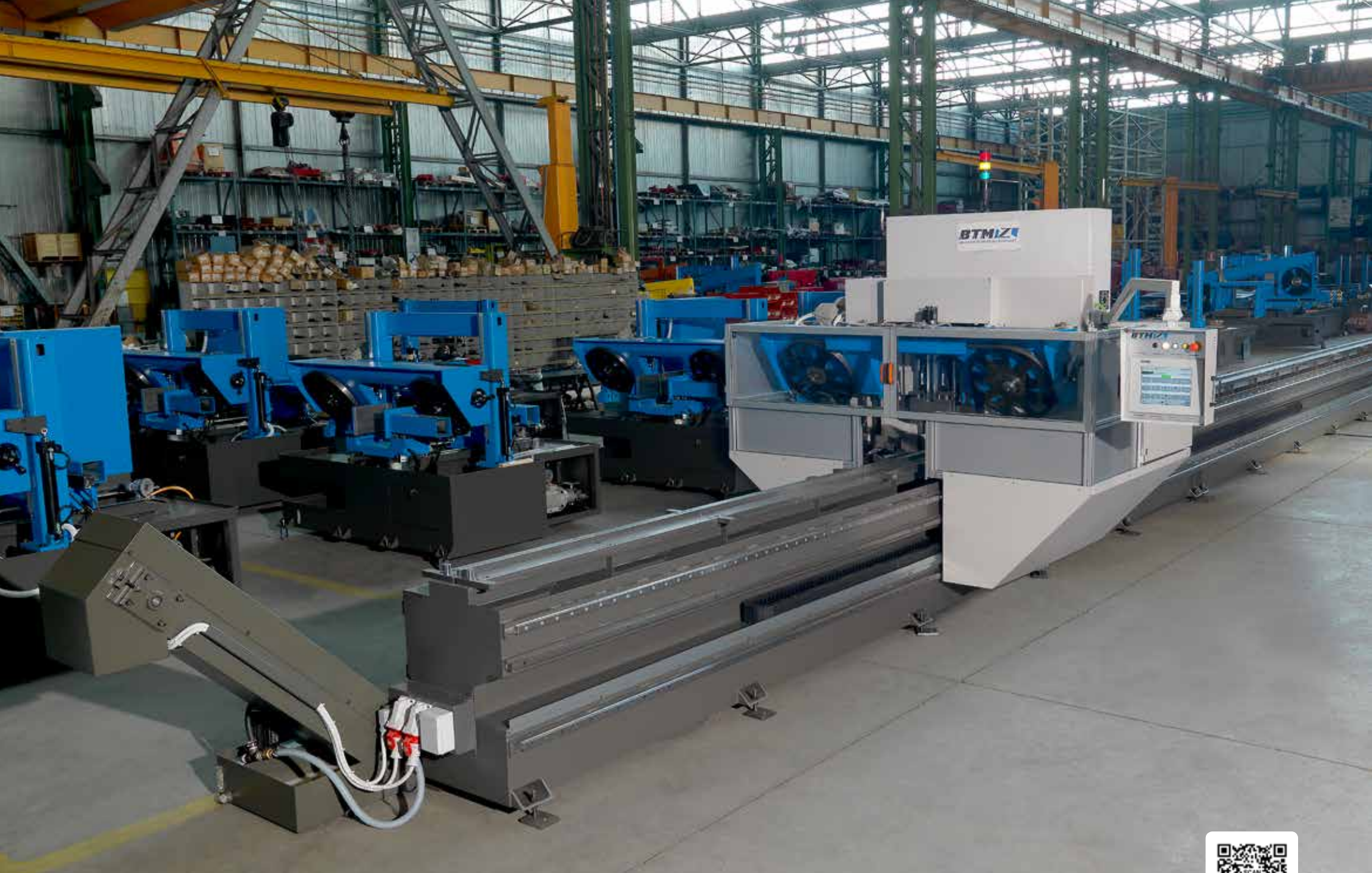
Impianto speciale per taglio e foratura binari Ø MAX 40 mm corsa 25 m Cutting and drilling system for railway tracks max ø 40 mm, carriage stroke 25 m
